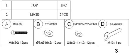
Step 1: Fasten the legs (2) To the top (1) with bolts (A), washer (B), spring washer (C) and using spanner (D)
